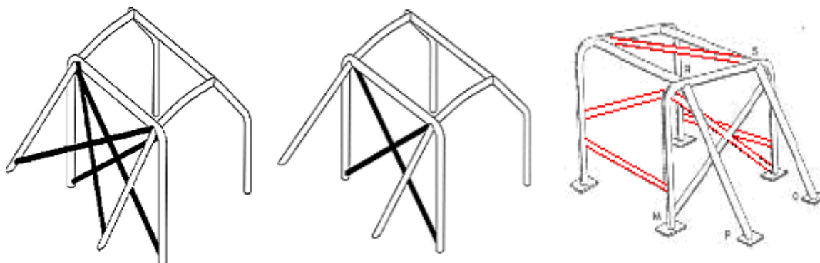
Figure G3: Suggested additional roll cage structural supports to be accepted by the Scrutineering Officer
